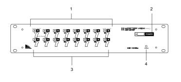
The figure shows a CS-1016 model. The only difference between it and the other models is in the number of Port Selection Switches.
