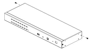
2. Use the M3 x 8 Phillips hex head screws supplied with the rack mounting kit to screw the rack mounting brackets into the sides near the rear of the unit.
