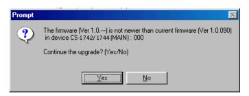
If you didn't enable *Check Firmware Version*, the Utility installs the upgrade files without checking whether they are a higher level, or not.
