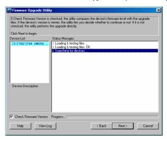
The Utility inspects your installation. All the devices capable of being upgraded by the package are listed in the *Device List* panel.
