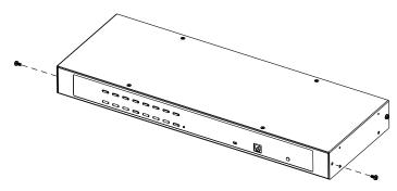
2. Use the M3 x 8 Phillips hex head screws supplied with the rack mount kit to screw the rack mounting brackets onto the side panels near the front of the unit.
