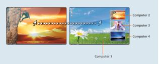
Cursor Shift Function – when you are using two displays, the mouse cursor can move back and forth across the displays, shifting the KVM focus.
