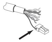
b) The second method is to use the STP cable shielding for grounding. In this case, make sure that the shielding makes tight contact with the top inside of the RJ-45 connector as shown in the diagram below:
